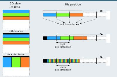
Data represent a two-dimensional array in the application (contiguous data along lines). Each color corresponds to a process/client.
